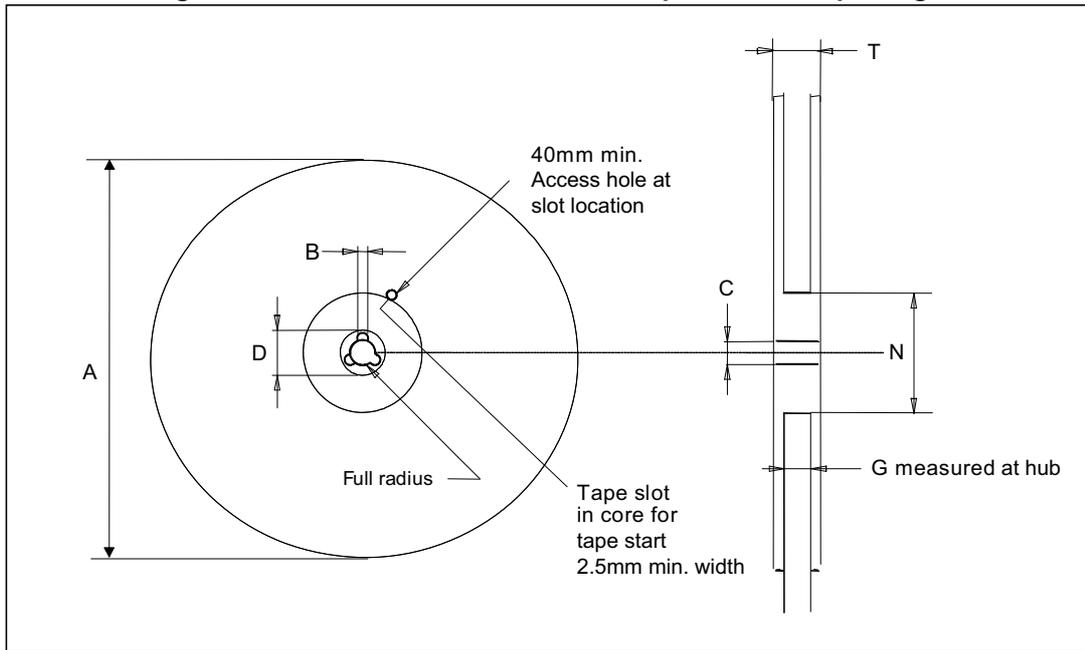
Table 87. Reel dimensions for carrier tape of LGA-16 package
