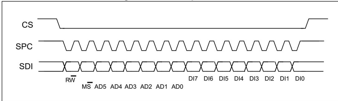
The SPI write command is performed with 16 clock pulses. A multiple byte write command is performed by adding blocks of 8 clock pulses to the previous one.
